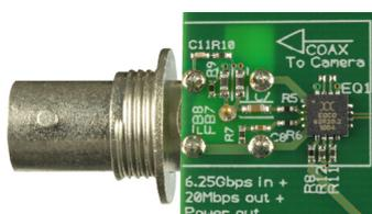
EqcoLogic have released their final silicon v1.0 transceivers as a physical layer solution for CoaXPress. This photo, shown here for interest, illustrates the compact physical size of the interface. (The connector is a standard BNC socket.)
